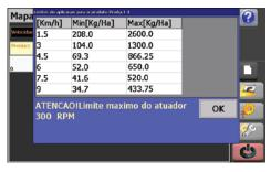
→ Rate table reports depending on speed to check whether the equipment is well-adjusted for the expected speed.
